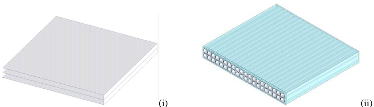
Figure 2. Geometrical configuration of AMR: (i) parallel-plates configuration and (ii): circular tube configuration
