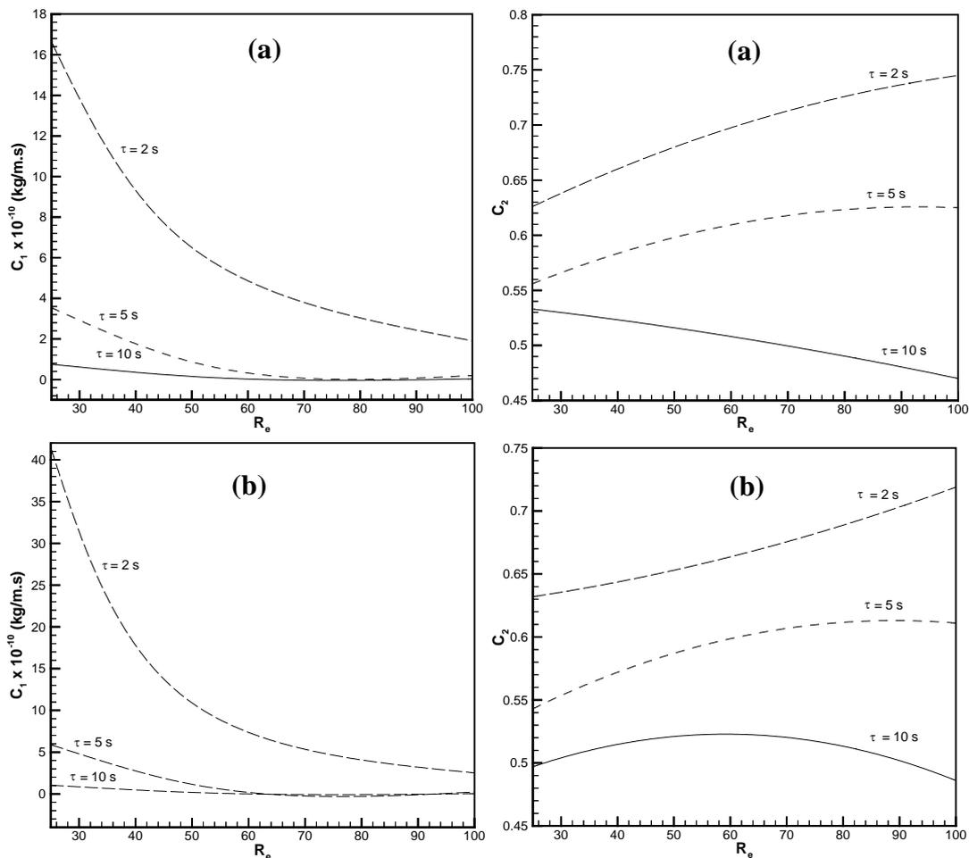
Figure 4. Coefficients  $C_1$  and  $C_2$  as function of Reynolds number, Re, and time period  $\tau$  for (a) parallel-plates configuration; (b) circular configuration
