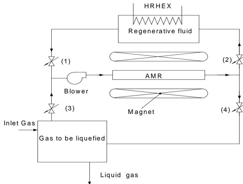
Figure 1. Schematic of principal of operation of AMR liquefier
