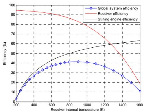
Figure 5. Efficiency versus the receiver internal temperature
