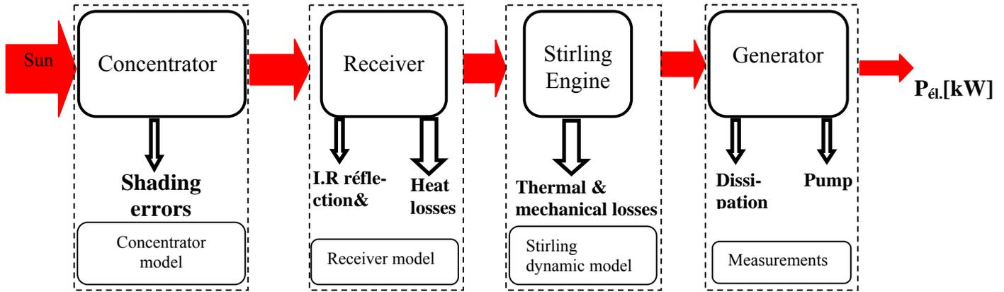
Figure 1. Schematic of Dish Stirling System solved in MATLAB
