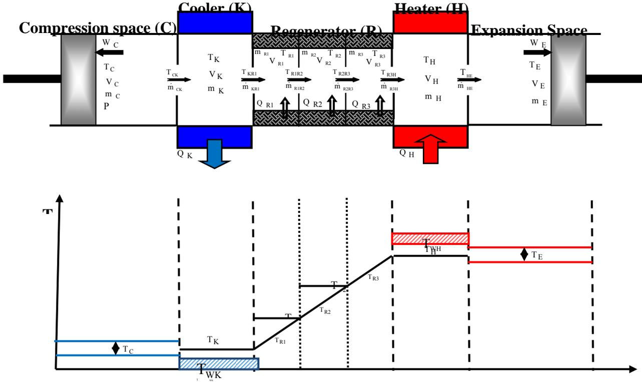
Figure 2. Stirling engine configuration and temperature distribution
