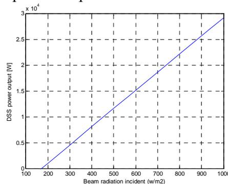
Figure3. Dish Stirling System power output
