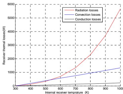
Figure 4. Heat losses in the receiver
