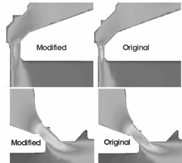
Figure 6. Velocity modulus fields obtained with the original geometry and the optimal modification.
