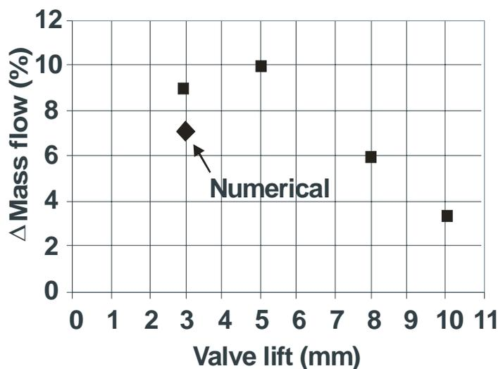
Figure 7. Mass flow increment attained for several valve lifts
