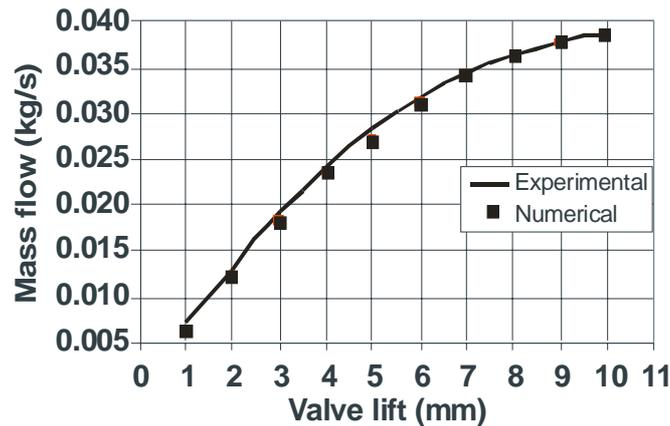
Figure 4. Comparison of experimental data and the predictions of the simulation for the mass flow obtained for a fixed pressure difference and different valve lifts.
