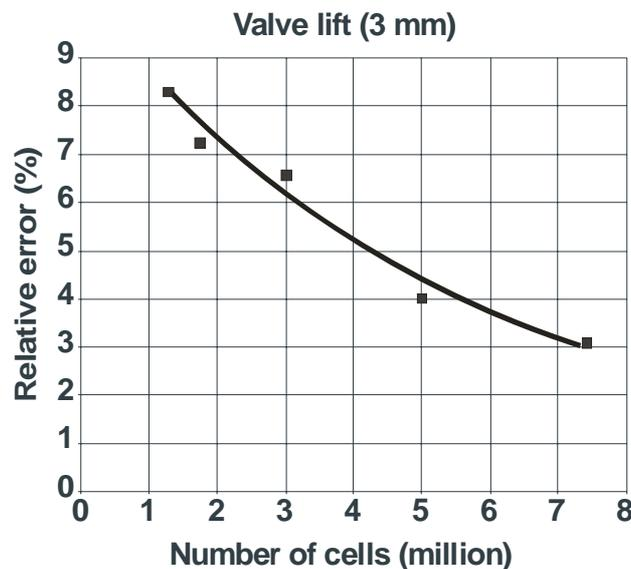
Figure 3. Error relative to the experimental value for a 3 mm valve lift.
