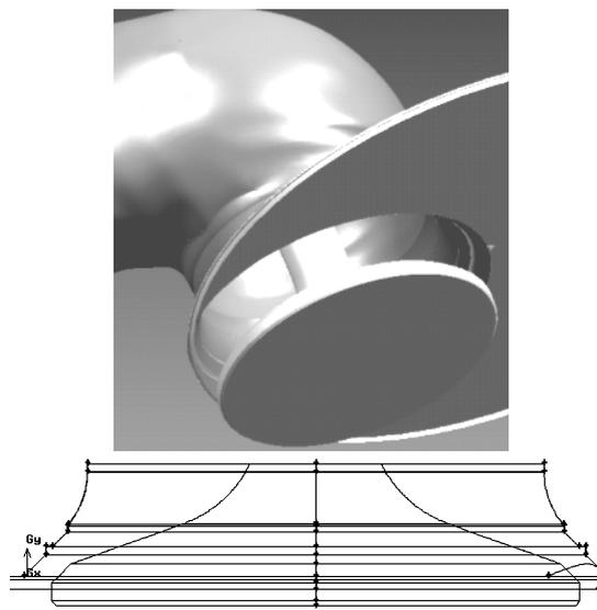
Figure 1. Details of the cylinder and the inlet manifold of the D909 engine.
