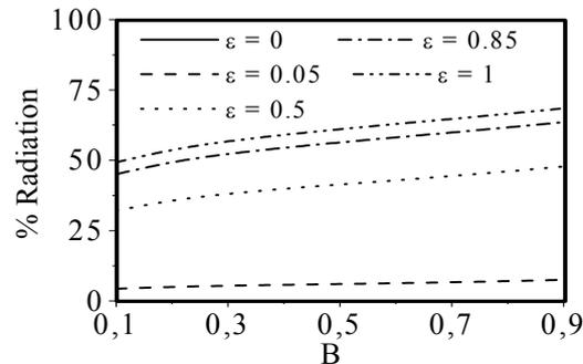
**Figure 4:** Radiation contribution to the global heat transfer versus  $B$ , for  $Ra = 10^6$  and various values of  $\varepsilon$ .
