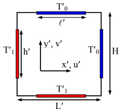
**Figure 1:** (a) Geometry of the problem with the imposed thermal excitations.
