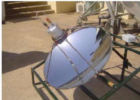
Fig 5: The solar spherical reflector used in the experiment [12]
