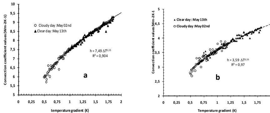
**Figure 3:** Convection coefficient values according to the temperature gradient during both measurement periods; (a): Convection coefficient values at the ground surface; (b): Convection coefficient values at the interior wall of the cover.
