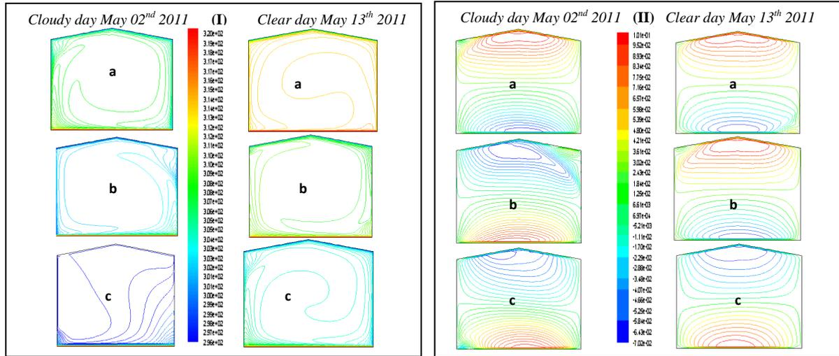
**Figure 2:** Temperature distribution (I) and horizontal component of the air velocity (II) in a vertical plane in the middle of the greenhouse at different instants (a): t = midday, (b): t = 6 pm, (c): t = midnight
