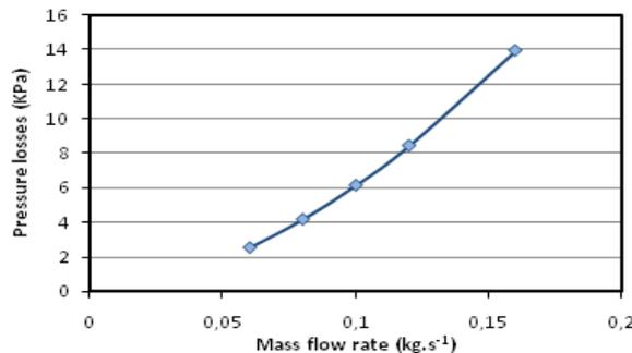
Fig.7: Pressure loss versus mass flow rate
