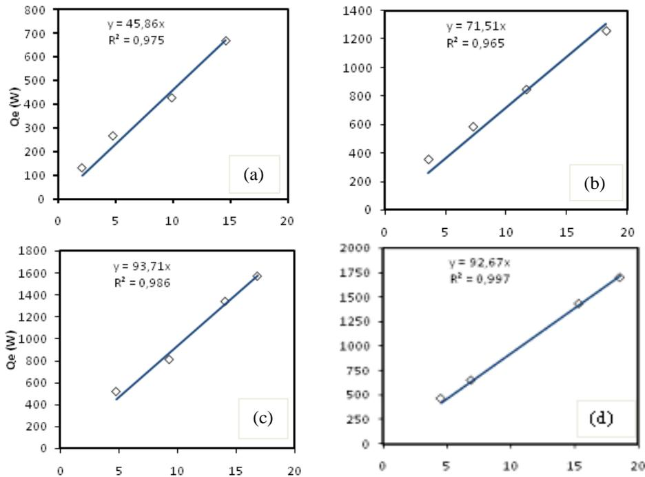
Fig. 4. Heat exchange rate versus log mean temperature difference for the following flow rates a) 0.06 kg.s<sup>-1</sup>; b) 0.08 kg.s<sup>-1</sup>; c) 0.1 kg.s<sup>-1</sup>; d) 0.12 kg.s<sup>-1</sup>.
