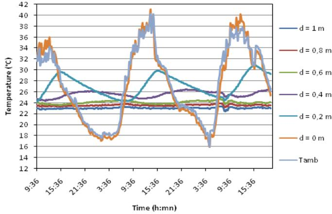
Fig. 2. Soil temperature at several depths 21-23 June 2011
