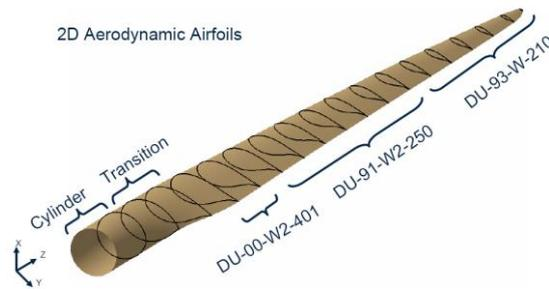
Figure 1 : Different Airfoils along the blade.
