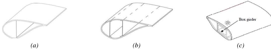
Figure 3 : Sketches of different blade concepts
