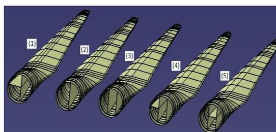
Figure 4 : Blades with different shear-web
