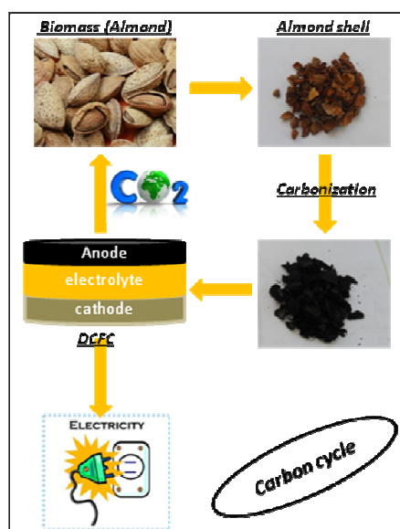
Figure 1: A clean and efficient integrated energy conversion system using almond shell biomass as fuel.
