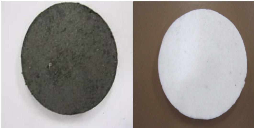
Figure 1: (a) 15% Graphite recycle+85%sel, (b) sel ( $\text{LiNO}_3$ )
