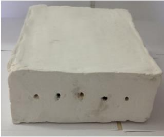
Fig1-b-: Composite: gypsum /copper tubes (12 mm outer diameter and 11.2mm inner diameter).
