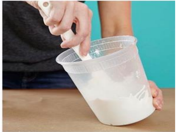
Fig. 2. Pasty mixture (gypsum + water).
