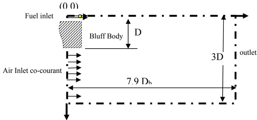
**Figure 1 Schematic of the combustion chamber ( $D_b=50\text{mm}$  and  $\phi_{\text{fuel inj}}=3.6\text{ mm}$ )**
