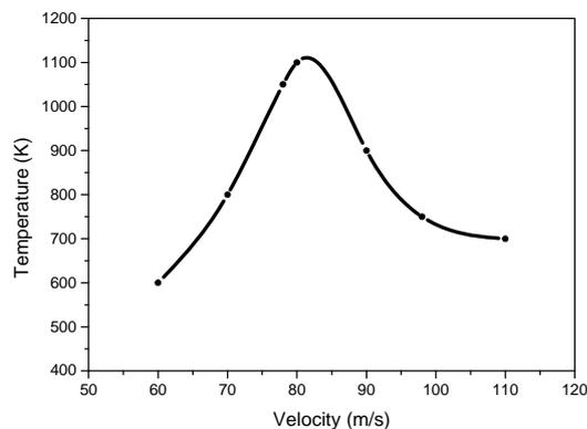
**Figure 5. Values of temperature results obtained with different velocities at an equivalence ratio  $\phi = 0.5$**
