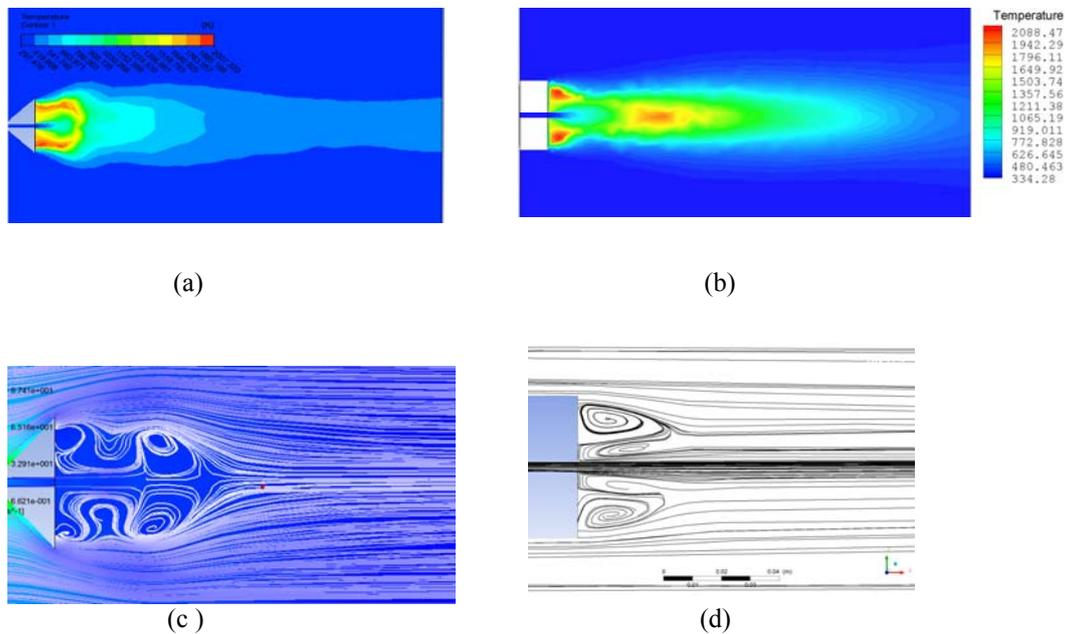
**Figure 7. Effect of the shape of the bluff body on the temperature contour and streamlines Triangular BB (a and c) , Cylindrical BB (b and d)**
