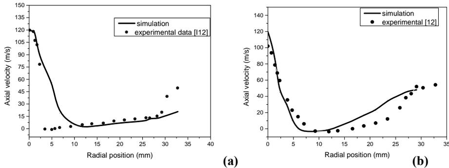
**Figure 3. Comparison between numerical and experimental results (a) at 3mm & (b) 30mm from Bluff Body**
