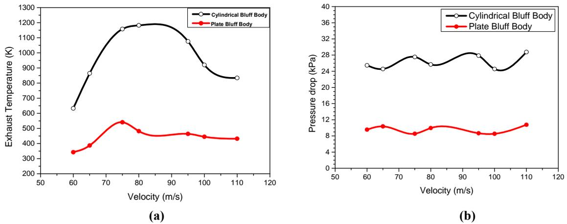
**Figure 6. Evolution of Exhaust Temperature (a) and pressure drop (b) with varying inlet velocity values for circular plate and solid cylinder as bluff body**
