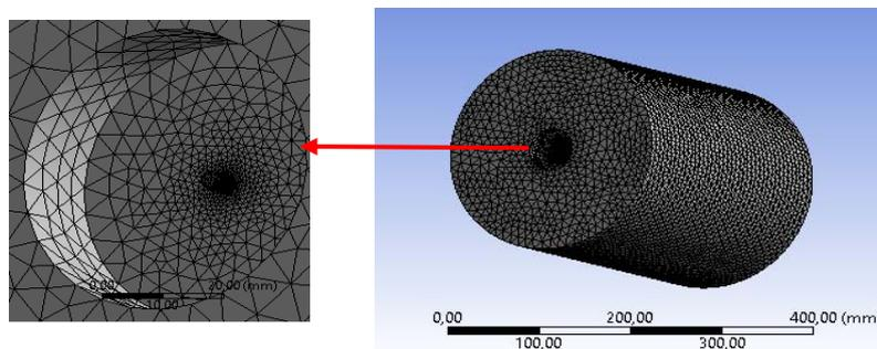
**Figure 2. Non uniforme Mesh of the combustion chamber (104876 elements)**
