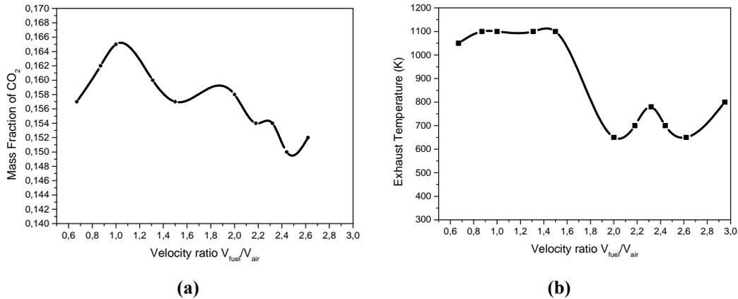
**Figure 4- Evolution of CO<sub>2</sub> mass fraction and exhaust temperature in function of velocity ratios at an equivalence ratio of 0.5**
