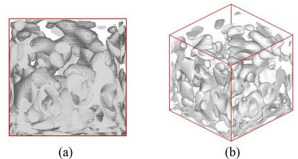
Figure 3: 3D slice (a) and isometric view (b) of an anisotropic porous medium by applying a dilatation gradient from -30% to +30% in vertical axis
