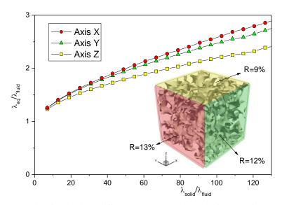
Figure 4: Nusselt number for the three-different axis x, y and z and their respective contact surface areas in an isotropic structure
