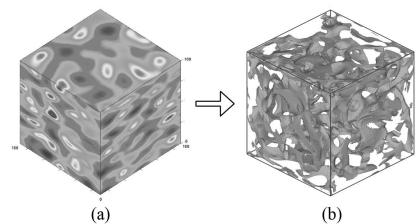
Figure 1: Development stages to generate a porous structure based on Gaussian random draws. Correlated Gaussian random field (a) and 3D structure 90% voids (b)
