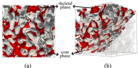
Figure 2: 3D slice (a) and isometric view (b) of an active and reactive wall in an isotropic porous medium with skeletal and coat phases
