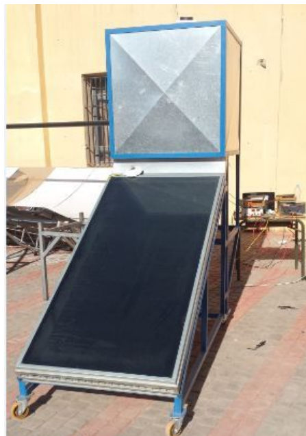
Figure 3: view of the experimental setup of the solar dryer
