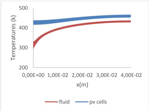
Figure 3: fluid and PV cell temperature vs channel length
