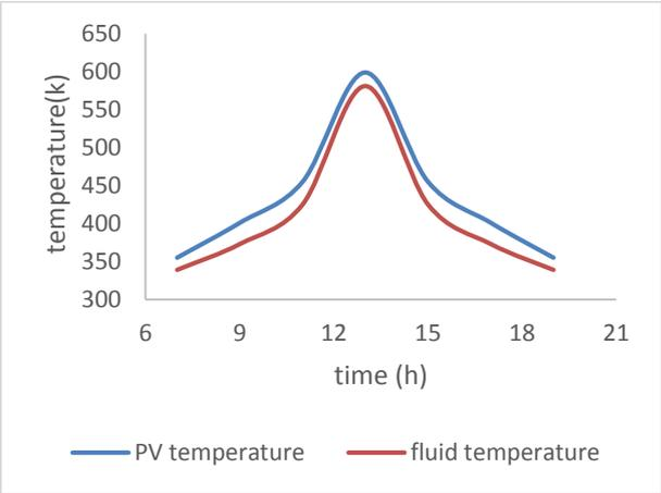
Figure 4: Temporal evolution of PV cell and fluid temperature of the CPV/T
