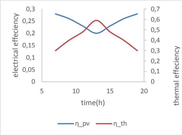
Figure 5: Temporal evolution of electrical and thermal efficiency of the CPV/T
