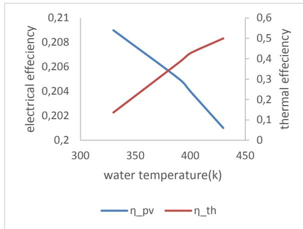
Figure 6: CPVT thermal and electrical efficiency vs fluid temperature.
