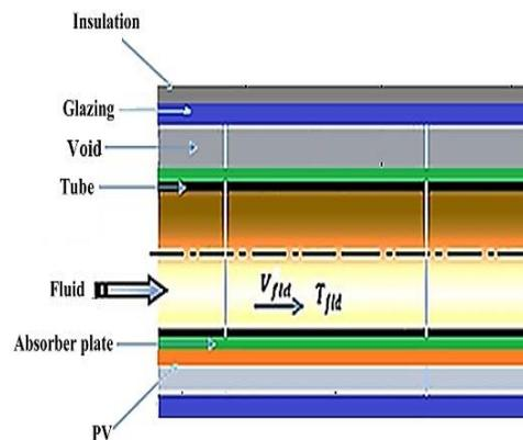
Figure 1 : CPV/T receiver layers
