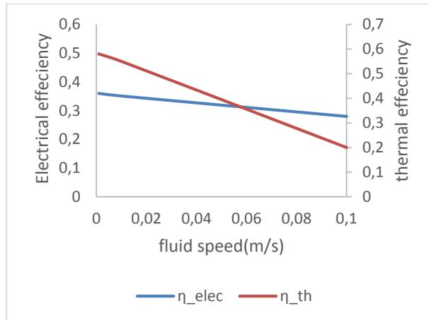
Figure 8: CPVT thermal and electrical efficiency vs fluid speed
