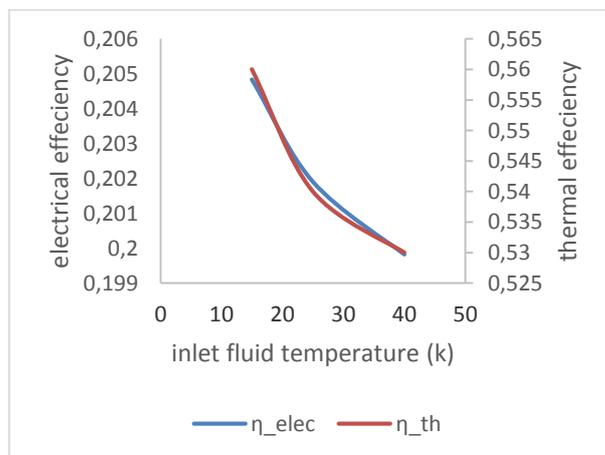
Figure 9: CPVT thermal and electrical efficiency vs inlet temperature.
