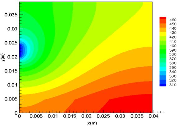
Figure 2: CPV/T layers temperature vs channel length
