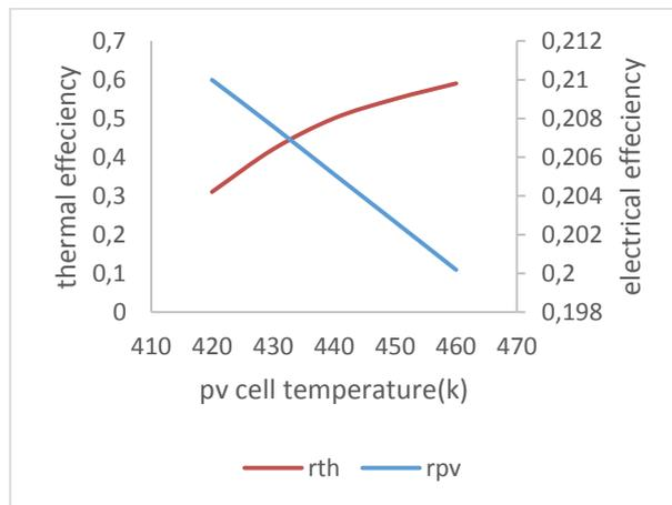
Figure 7: CPVT thermal and electrical efficiency vs PV cell temperature
