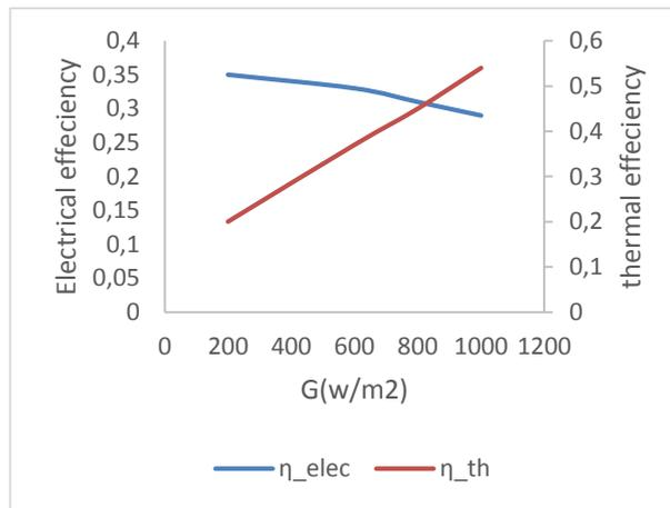
Figure 10: CPVT thermal and electrical efficiency vs beam radiation
