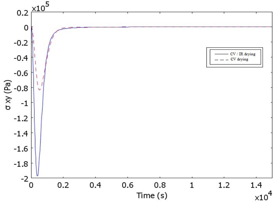
Figure 5 : The variations of stress  $\sigma_{xy}$  versus drying time obtained for convective drying at different sample positions ( $T_a = 60$  °C,  $RH = 23$  %,  $P_{IR} = 800$  W/m<sup>2</sup>)
