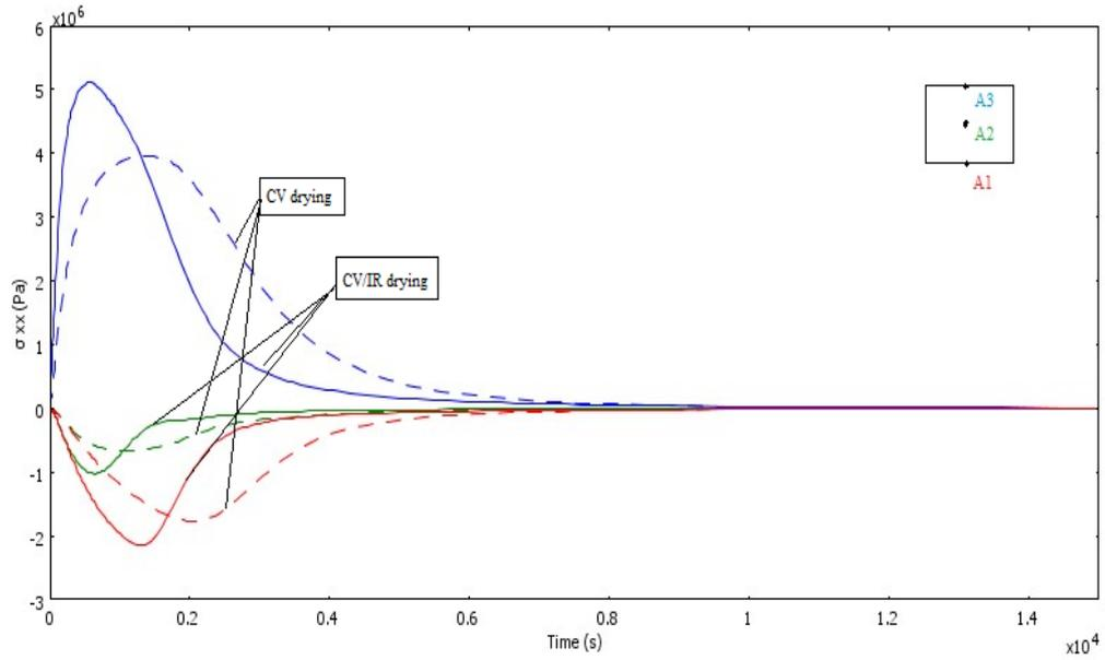
Figure 3 : Variations of stress  $\sigma_{xx}$  versus drying time at different sample positions ( $T_a = 60\text{ }^\circ\text{C}$ ,  $\text{RH} = 23\%$ ,  $P_{\text{IR}} = 800\text{W/m}^2$ )
