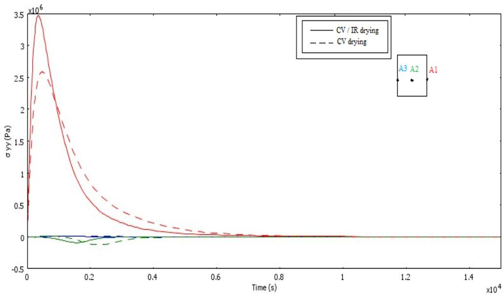
Figure 4 : Variations of stress  $\sigma_{yy}$  versus drying time at different sample positions ( $T_a = 60\text{ }^\circ\text{C}$ ,  $\text{RH} = 23\%$ ,  $P_{\text{IR}} = 800\text{W/m}^2$ )
