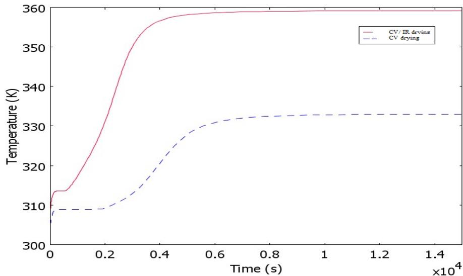
Figure 2 : Temperature distribution at the surface of the Bovine leather
